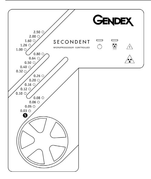
Power on the system by the mains switch. Green mains lamp O must light up, the timer is in stand-by mode.
